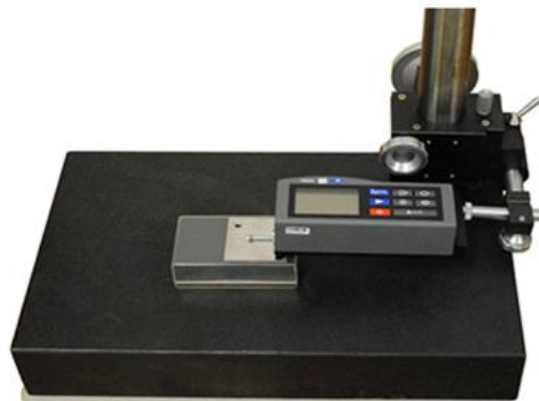
Figure 5: The surface roughness measurement on a specimen using surface tester TR 200
